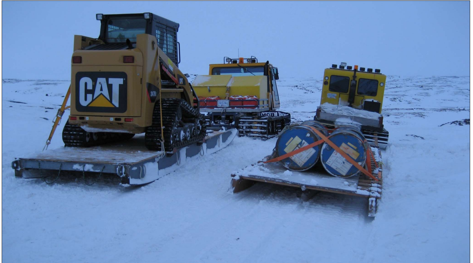
A Caterpillar® Multi-Terrain Loader was mobilized to Chidliak overland in May 2009 using Bombardier Sno-Cats.
